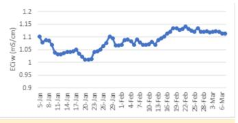
**Figure 3.** Daily average of irrigation water EC collected with ES-2 sensor.
