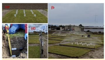
**Figure 2.** Catch cans used for irrigation uniformity test (a), uniformity test at the plots (b), TEROS 12 sensor during installation (c), and setup for continuous canopy spectral and temperature data measurements. (d).
